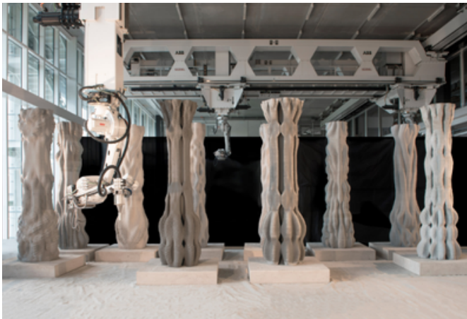
Image 14. 3D printed complex concrete structures (Source: de zeen)
